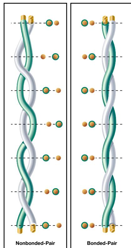
Nonbonded pairs can lose the uniformity of twist that is essential to consistent electrical performance.
